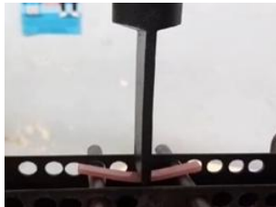
Figure 4. Sample testing using the Universal Testing Machine 3-Point Bending technique. (Source: Personal Documentation)
