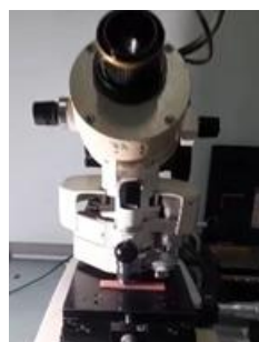
Figure 2. Surface hardness testing on samples using a Vickers Hardness Tester (Source: Personal Documentation)
