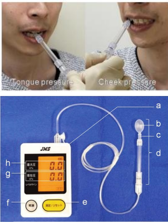
Gambar 2. Pengukuran kekuatan tekanan lidah ( JMS tongue pressure measurement device ®): (a) digital tongue pressure measurement device; (b) balloon (width: 18 mm, height: 25 mm); (c) plastic pipe (width: 6 mm, height: 10 mm); (d) disposable probe; (e) measurement/reset; (f) power; (g) present pressure; (h) maximum pressure. 16
