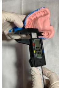
Figure 3. Measurement of Impression Results Using a Digital Caliper
