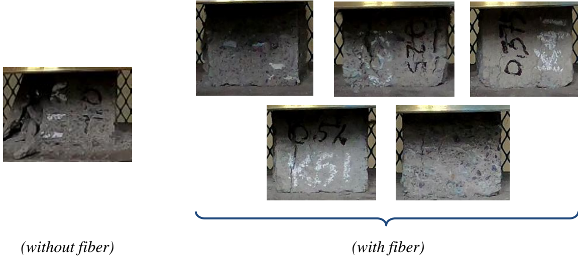
FIGURE 9. Compression strength test failure rate
