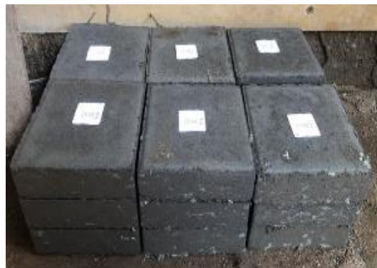
FIGURE 7. Whole block paving test object
