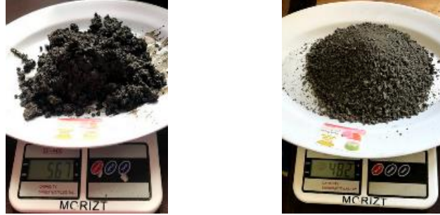
Figure 2. Pictures of sand (left) and stone ash (right)
