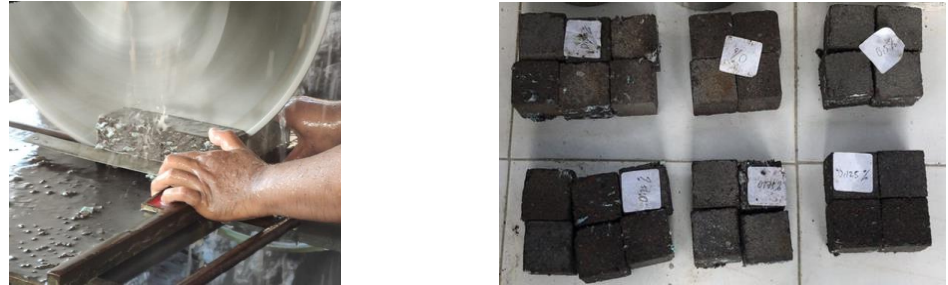
FIGURE 7. The paving cutting process and the shape of the paving block cube test object
