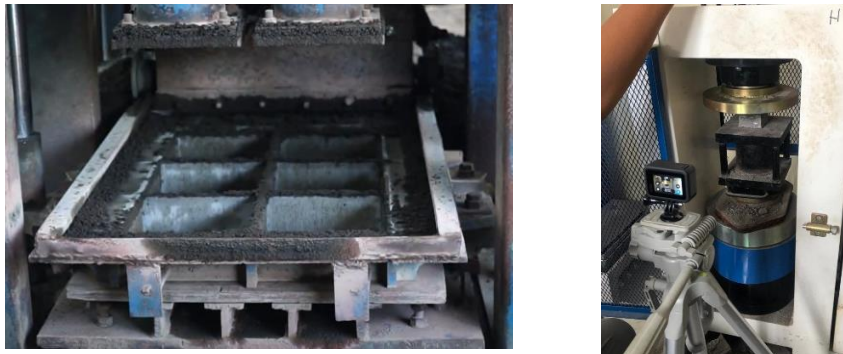
Figure 3. Specimen mold (left) and universal test equipment (right)
