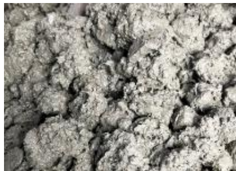
FIGURE 4. Mask fiber concrete mixture
