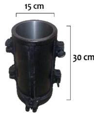
FIGURE 2. Specimen mold (left) and universal test equipment (right)
